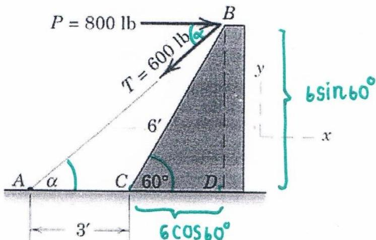
$$\begin{aligned} \rightarrow R_x &= 800 - 600 \cos \alpha \\ &= 346.5 \text{ lb} \end{aligned}$$
